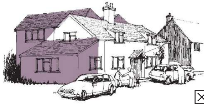
Figure 8.7: Extensions which are larger than the parent building can harm the appearance of the original house
