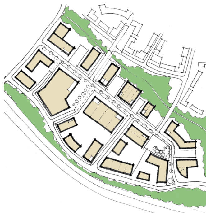
Figure 5.29: Layout plan showing indicative block layout with frontage and entrances overlooking the boulevard
