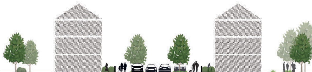
Figure 5.21: A good formal arrangement for a primary street that incorporates parallel parking with regular tree planting within kerb build outs reducing its impact on the street space (Section)
