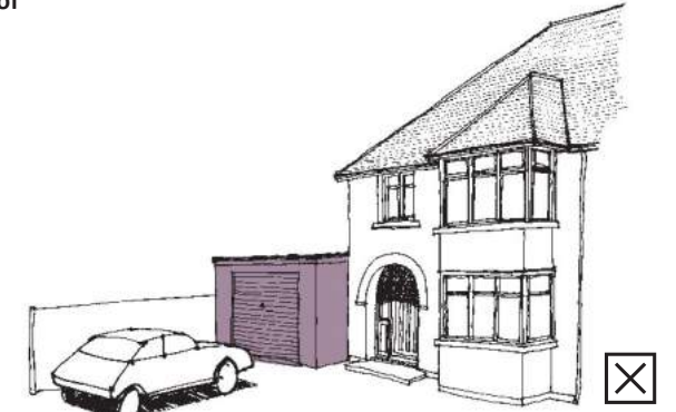
Figure 8.38: Garages which are forward of the main building line and of dissimilar shape are unlikely to receive permission
