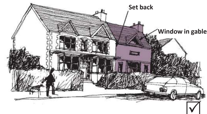
Figure 8.5: A lower, set back extension which repeats the overall shape and design of the house
