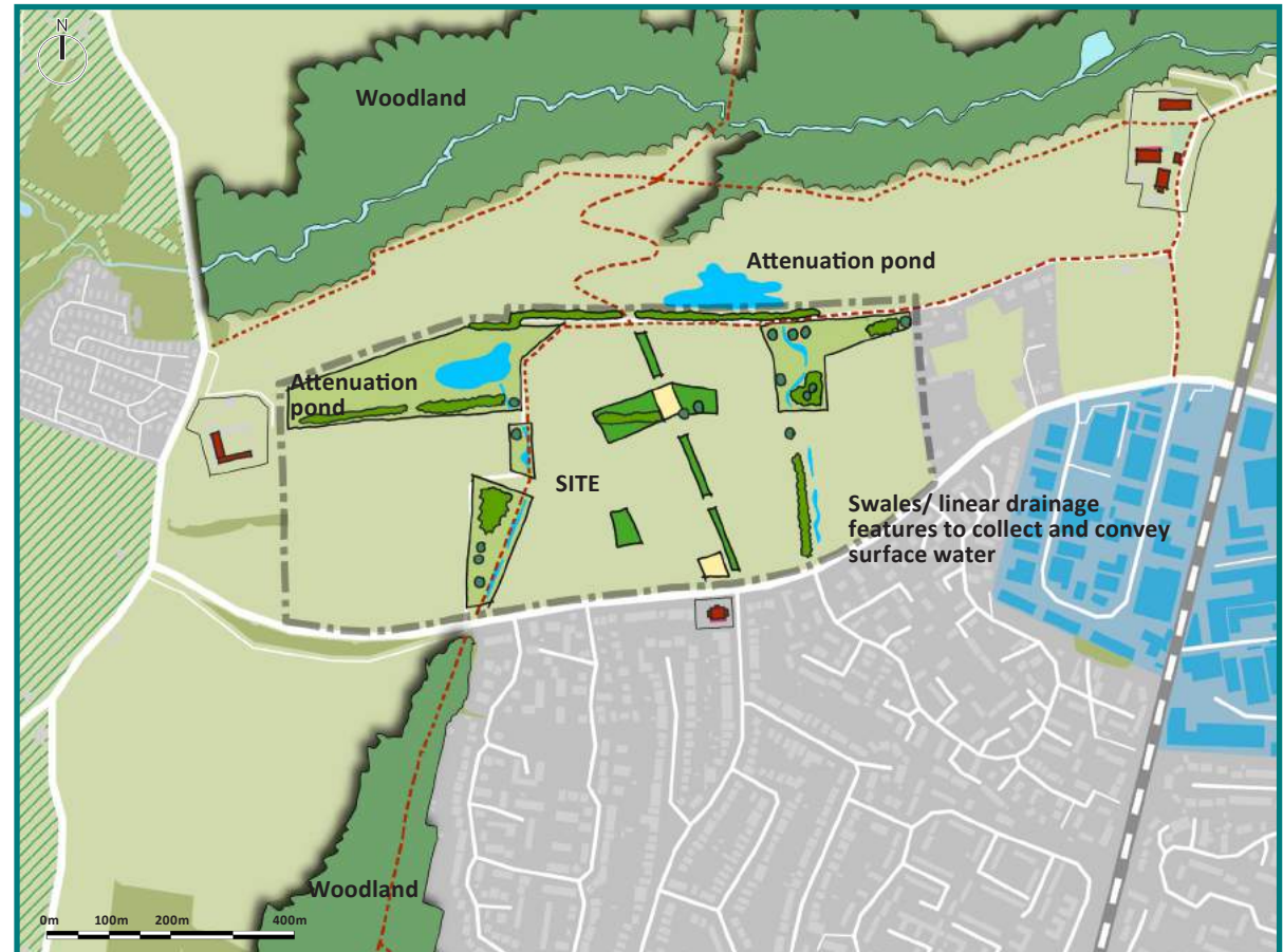
Figure 4.3: INDICATIVE SITE CONCEPT PLAN 3 - A sustainable drainage network incorporated within open spaces is proposed through the site
